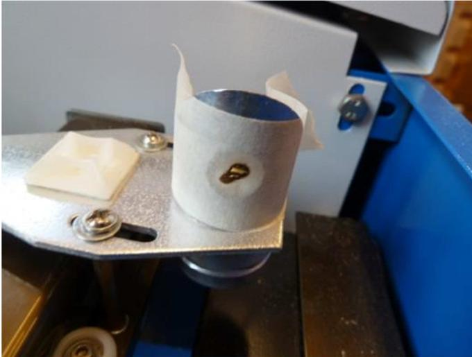
The last stage of the alignment process is to ensure the lens holder is straight. Remove the angled mirror from the top of the holder and place a piece of tape over the hole. Remove the tap from the front.
