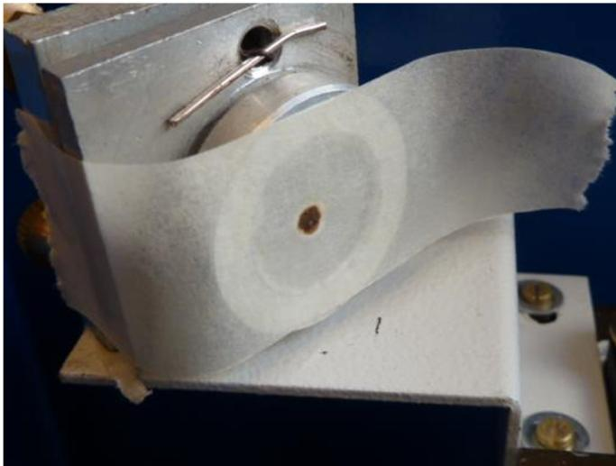
A well-adjusted fixed mirror and correctly positioned Y axis mirror will give a result as above. Once this has been achieved the Y axis mirror can be aligned.
