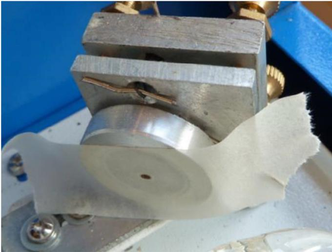
Once the mirror is positioned, ensure all the screws are tightened, remove the masking tape and clean the mirror to remove the burnt residue of masking tape.
