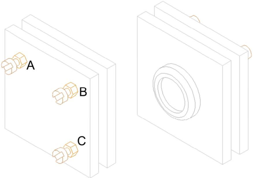
The picture above shows mirror adjusting assembly. The three screws A, B & C are locked with lock-nuts. These should be treated with care - the screws and nuts are brass and have a fine pitch thread. Too much enthusiasm will result in stripped threads probably requiring a new mirror assembly.
