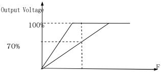
Auto energy saving can reduce the normal output voltage by max 30%. For the load with frequent changes or closing to full load, this function is not suitable.
