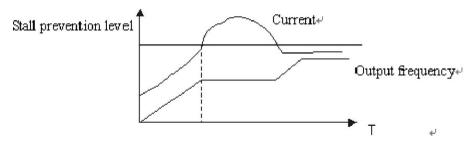
100% current is the rated current of the motor. When this parameter is set to 0, the stall prevention function is invalid.
