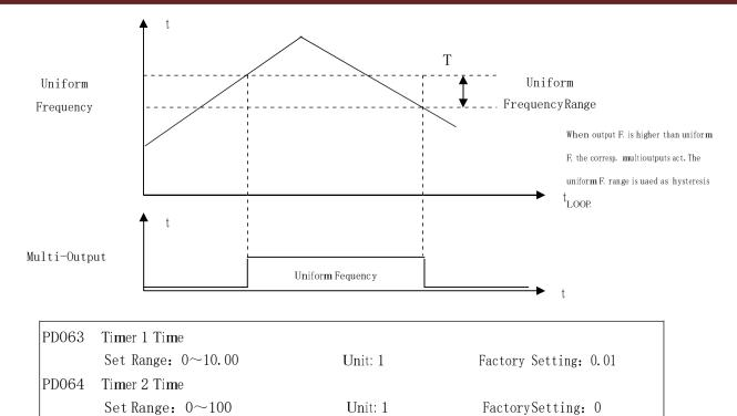
Timer 1 is a timer of 0.1s  $\sim$  10.0s and Timer 2 is a timer of 1s  $\sim$  100s. When the timer start at multi-inputs is closed (on) the timer starts to count time. When it reaches the set time the corresponding multi-output contact will act. When the timer start is opened (off) the timer time at the multi-output will be reset.
