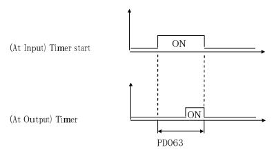
For example, set PD063=5.0s. When the external control terminal (Multi-Input) is valid the output terminal will be valid after five (5.0) seconds, the signal of which can be used to control other corresponding signals.
