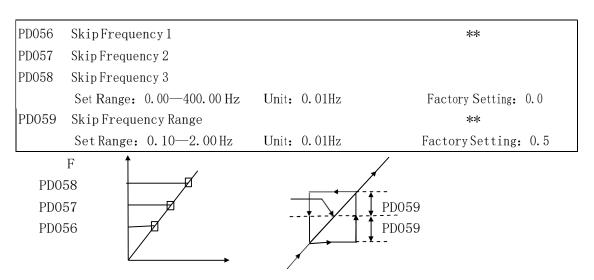
These three frequency skipping points are set for avoiding a mechanical resonance point. In case of PD059=0, all skip frequencies are invalid. The actual skip frequency range is two times that of PD059, as shown in the above diagram
