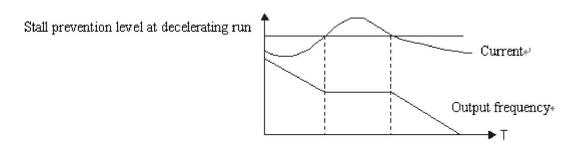
100% current is the rated current of the motor.
