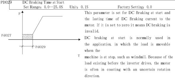
So the DC braking can be executed before starting the motor to prevent the inverter from tripping. This setting is valid only when PD025 is set to 0. For the related parameters refer to PD025, PD031 and PD027.
